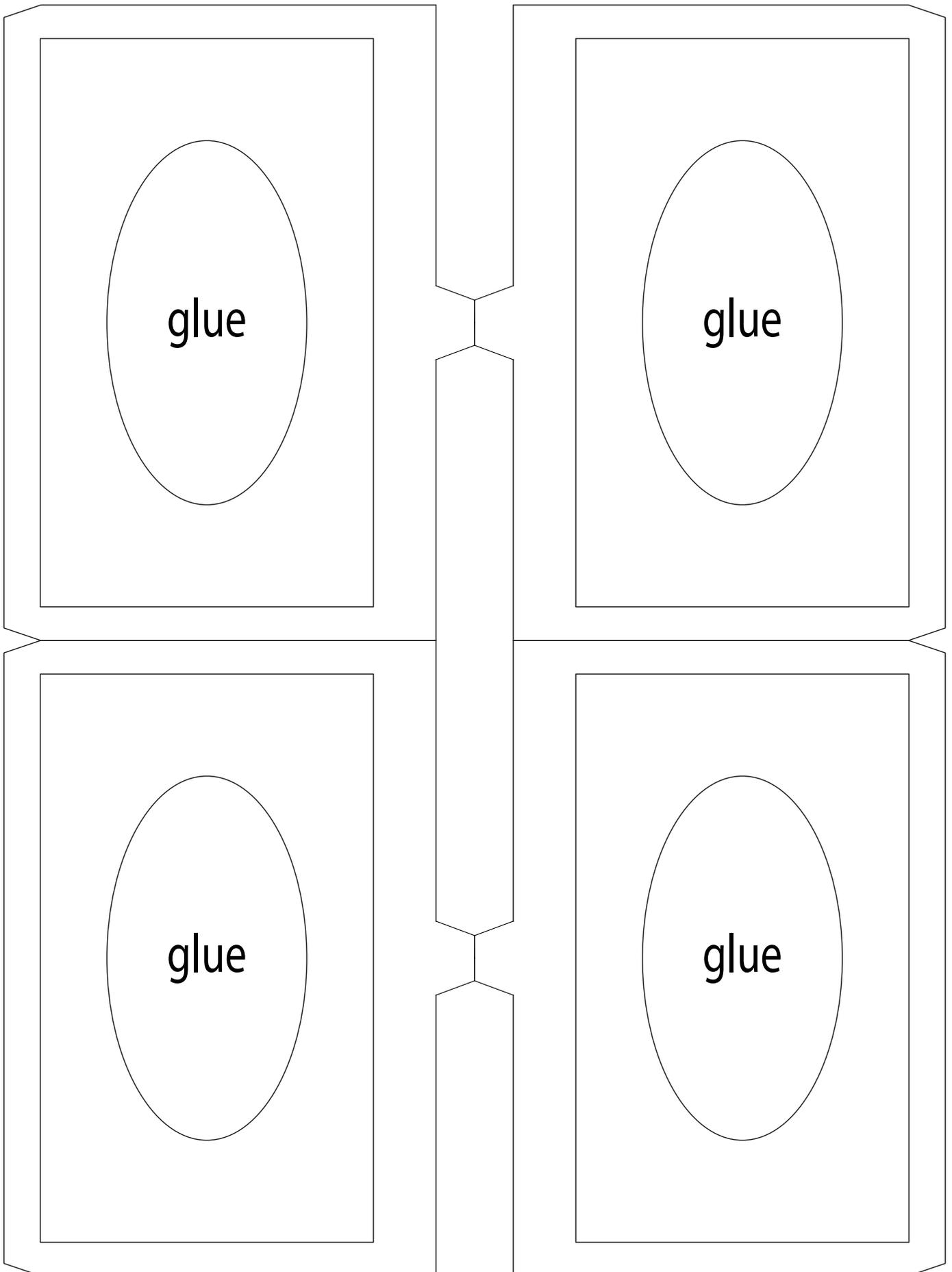
Glue marked positions to black 270 g/m<sup>2</sup> cardboard, cut outer lines, then cut hole for image.
